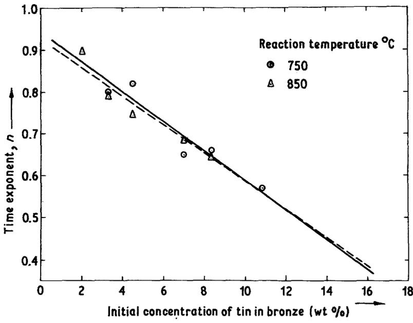
Figure 4 Variation of time exponent  $n$  with the initial tin in bronze at 750 and 850°C.
