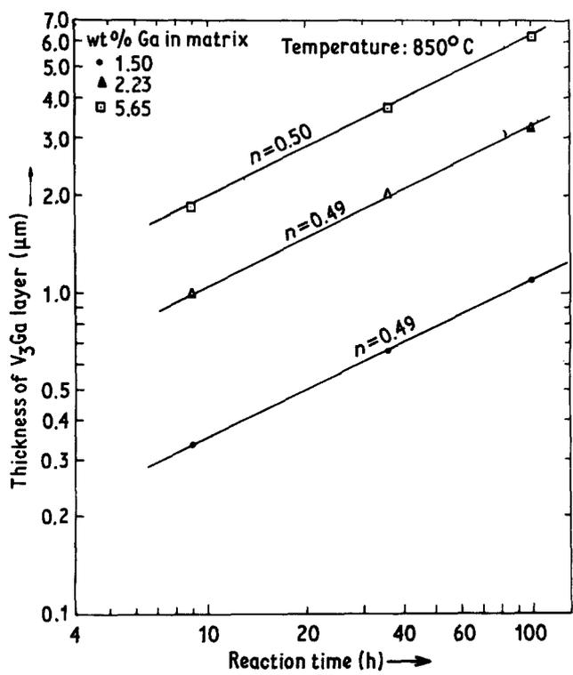
Figure 5 Log  $R$ -log  $t$  plots at 850°C for different concentrations of gallium in bronze.
