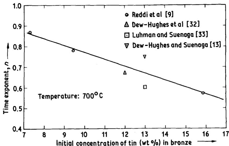
Figure 3 Variation of time exponent  $n$  with the initial concentration of tin in bronze at 700° C.
