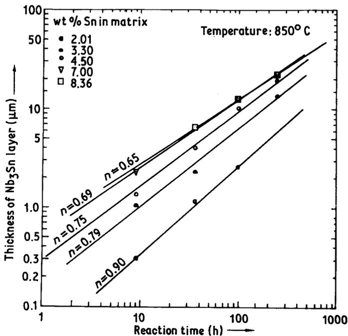
Figure 2 Log  $R$ -log  $t$  plots at 850°C for different concentrations of tin in bronze.
