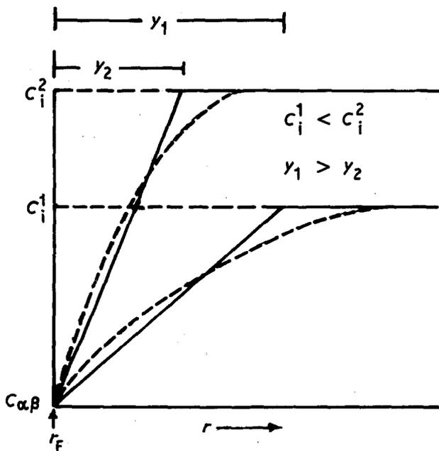
Figure 8 Schematic dependence of the effective diffusion distance with the initial concentration  $c_i$ .
