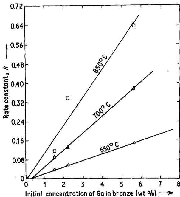
Figure 6 Variation of the rate constant  $k$  as a function of gallium concentration for three reaction temperatures.
