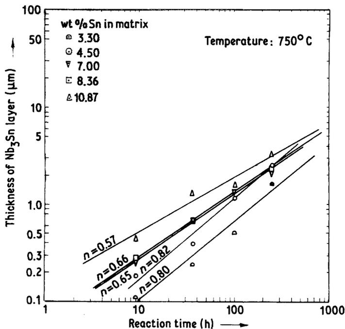
Figure 1 Log  $R$ -log  $t$  plots at 750°C for different concentrations of tin in bronze.
